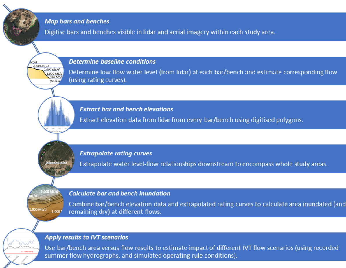
Figure 3. Flow diagram summarising the analysis approach used to assess bar and bench inundation.
