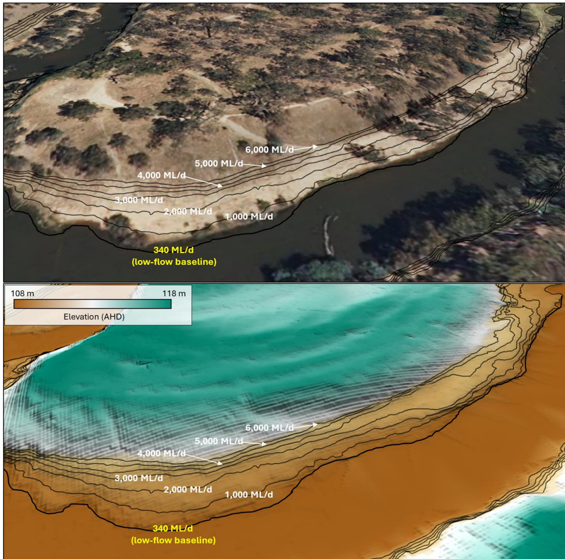
Figure 5. Simulated inundation at Oval Bend Camping Area under flows ranging from 340–6,000 ML/d. The site is within the Moss Road study area.
