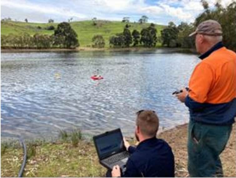
Figure 3. Utilizing remote controlled bathymetric instrumentation to accurately set the siphon intake level ensuring the siphon breaks at the identified water security level (a hard fail-safe)
