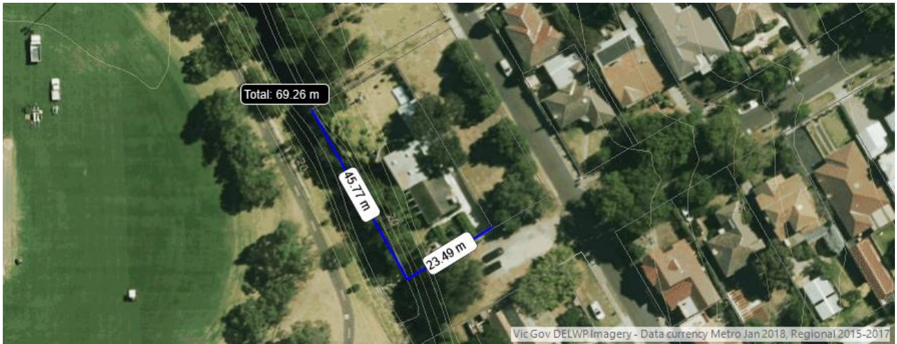
Figure 1 A property on banks of an urban stream. The contours show that the house is at the top of bank and that there is essentially no setback (Source: Vicplan).
