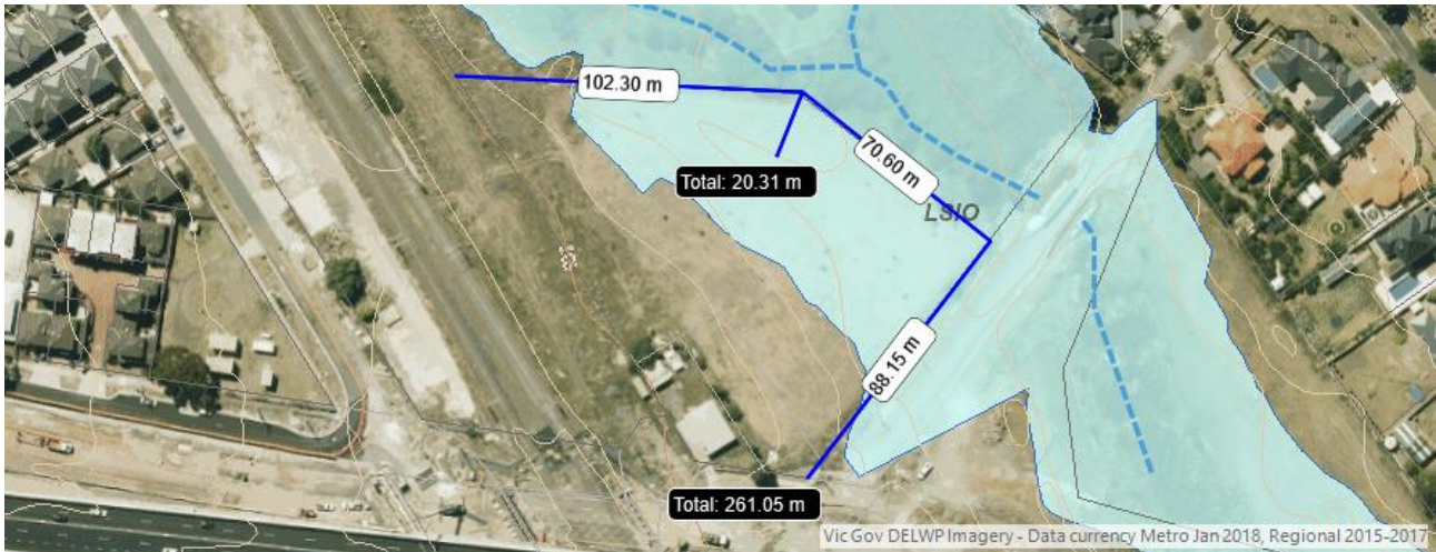
Figure 3 Land Subject to Inundation Overlay is demonstrating that much of this property is subject to flooding, and that despite it being in an urban area, a setback of 20m or more would be easily achievable. (Source: VicPlan)
