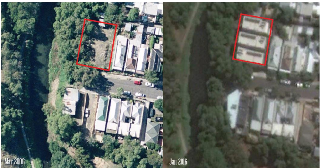
Figure 2 Development has been allowed to occur at the top of bank (left), enabling another development to use this precedence and be located with a similarly inadequate setback 10 years later (right). (Source: Google Earth Pro).
