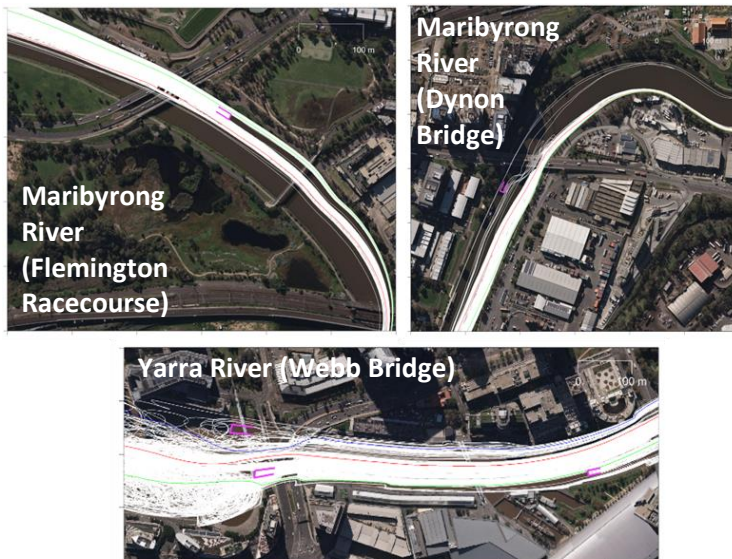
Figure 5. Particle track modelling outputs showing litter pathways (white) in relation to the positioning of the Bandalong traps (magenta rectangles)
