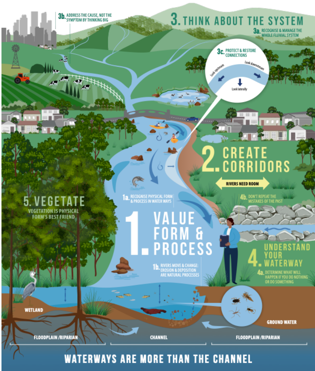
Figure 1. Overview of the Physical Form Five principles as they relate to waterway and catchment management that considers geomorphic theory and working with waterways (Diagram developed by Streamology and Ooid Scientific).
